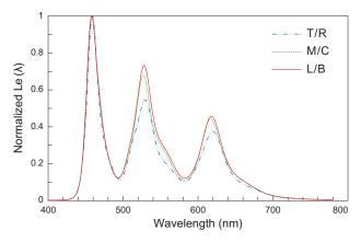
Fig. 2 Spectra of an OLED display at RGB output signal level [19/19/19] at different display positions.
