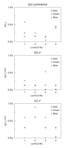
Fig. 7 Measurement accuracy of LumiCol 1900 (for color). The deviations from spectroradiometer measurements with respect to luminance and chromaticity were determined on a display showing colored images (red, green, and blue represented by circles, squares and triangles respectively).
