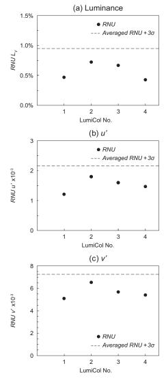
Fig. 8 Response non-uniformity of four different LumiCol 1900 devices determined from measurements on a uniform light source with a luminance level of 100 cd/m<sup>2</sup> (represented by symbols). The *RNUs* were determined for the quantities luminance (a) and color coordinates u' and v'. The dashed lines mark the  $ave+3\sigma$  values.
