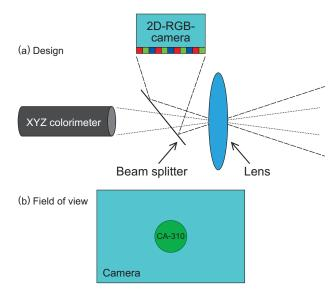
Fig. 5 Design and field of view of LumiCol 1900.
