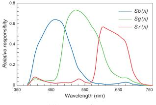
Fig. 4 RGB camera spectral responsivity.
