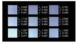
Fig. 1 Example of uniformity inspection. View of OLED displays. Each display image is at RGB output signal level [19/19/19]. Where Lv denotes luminance value, and u' and v' denote color coordinates.
